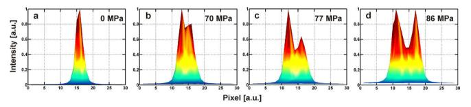
Fig. 5. (1 3 1)-Peak splitting during loading prior to the "Laue yield" for the 8 µm Ni-B pillar, showing that the "Laue yield" is still an overestimation of the onset of plasticity.
