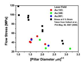
Fig. 7. Hall–Petch plot showing the "Laue yield" for all 10 Au samples as a function of the square root of the diameter. Black squared data points are taken from Ref. [6] and were derived at 5% strain from stress–strain curves of single slip oriented Au pillars.
