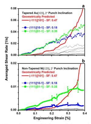
Fig. 6. Average shear rates on all 12 slip systems for the compression of micropillars of the same geometry and taper as investigated in the current experiments. The boundary conditions were compression at zero friction and tool inclination of  $2^{\circ}$  off the ideal punch direction (SF, Schmid factor). (a) Tapered Au pillar and (b) non-tapered Ni pillar.
