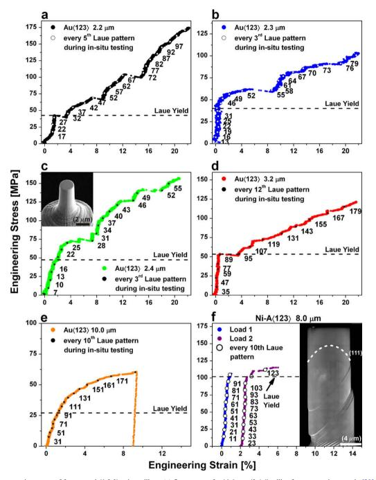
Fig. 1. (a–d) Stress–strain curves of four tested  $\langle 1 2 3 \rangle$ -micropillars, (e) flow curve of a 10.0  $\mu$ m  $\langle 3 4 6 \rangle$ -pillar from a previous study [29], and (f) an load–unload test performed on the 8.0  $\mu$ m Ni-A $\langle 1 2 3 \rangle$ -sample. The inset in (c) displays the undeformed pillar, and the deformed Ni-A is depicted as an inset in (f).
