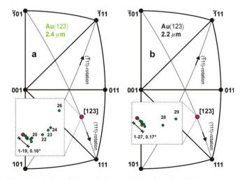
Fig. 4. Evolution of the vertical crystal axis orientation for the 2.4  $\mu m$  (a) and 2.2  $\mu m$  (b) Au(1 2 3)-sample, revealing initial activation of the (1 1 1)-plane. In both cases the corresponding Laue pattern numbers and the total amount of rotation are indicated.
